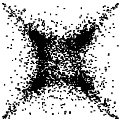
Fig. 5.4. Wehner spots predicted for 3 keV Ar bombardment of Ni(100). The limits of the plot correspond to p_z = 0 , or \varphi = 0^\circ , while the origin represents \varphi = 90^\circ (normal emission). The directions of preferential emission (diagonals of plot) are parallel to \langle 001 \rangle surface rows.
